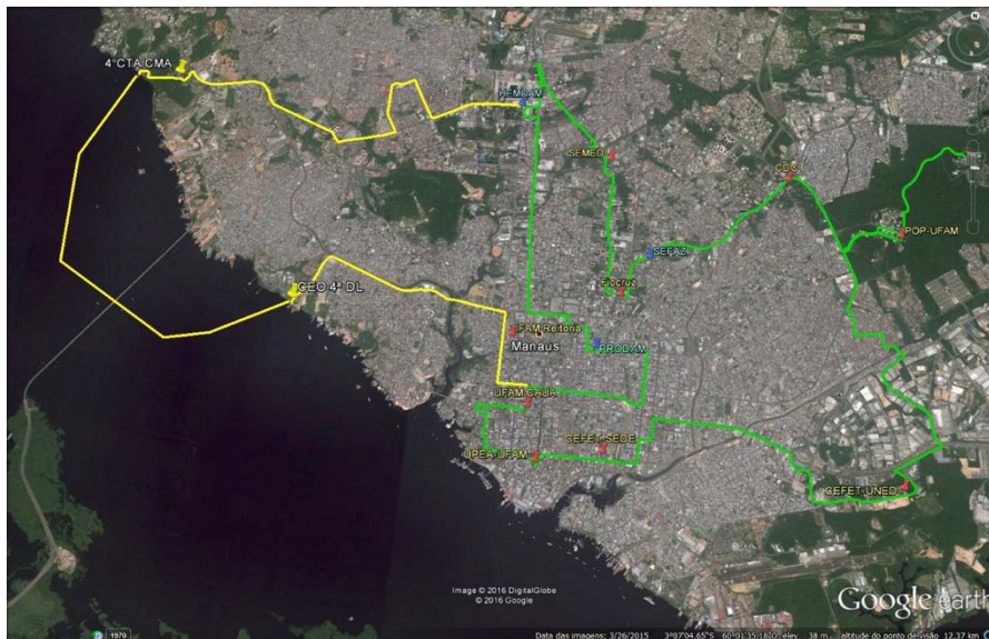
Fig. 17 The 6,800 m subfluvial cable deployed in the River Negro in Manaus
